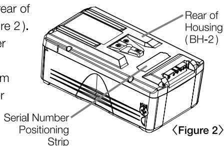
**Caution : The ELITE battery pack will not charge or discharge if different serial number Power Cartridges are used and a warning LED code will show.**
