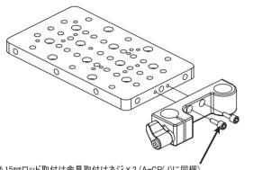
$\phi$  15mmロッド取付け金具取付けネジ×2 (A-CP(J)に同梱) Cheese Plate Support for  $\phi$  15mm Rod Screw x 2
