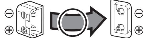
Please confirm the shape of connector and  $\oplus$   $\ominus$  polarity of plug side prior to connect with receptacle. Please do not force it when felt it is difficulty.
