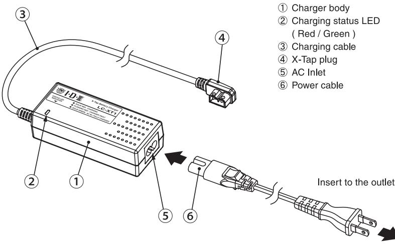
1 : Insert a plug into the battery equipped with X-Tap connector, and start charging.
