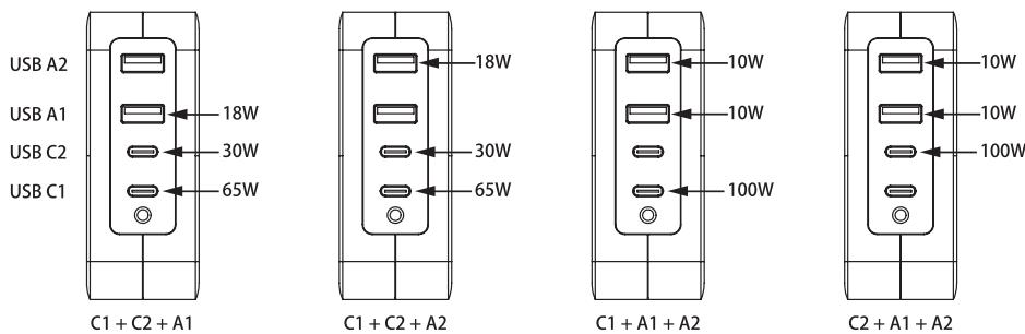
\* When using 3 or more ports with 2 USB-C ports in use, the maximum USB C1 is 65W and the maximum USB C2 is 30W.
