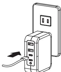
2. Connect the supplied USB Type-C cable into the USB-C port on the charger and the USB-C port on the IDX battery to start charging.
