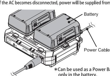
\*If the AC becomes disconnected, power will be supplied from the mounted batteries.
