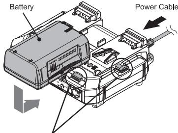
5 : When removing the battery from the charger, firmly press the release button while lifting the battery straight up.
