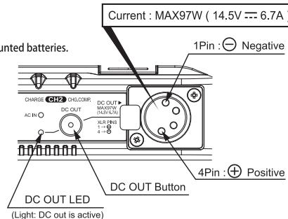
\* Please ensure that the mounted batteries meet the power requirements for the device connected (MAX DC output is 97W/6.7A).
