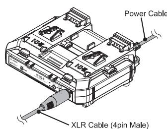
◎ When used as an uninterruptable power supply
